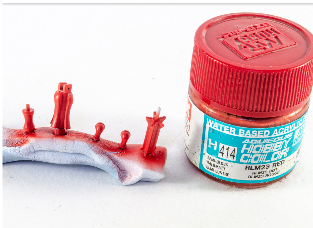
156. Take all your brass and 3D printed parts (not all shown here) and prime them before painting in your chosen colour. Our prototype used red paint.
