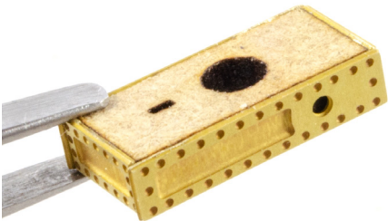
171. Now glue the side parts into position. These are parts #PE-31 and #PE-32. The orientation of these is very important. Use these photos and the plan to confirm you have this right. When complete, gently sand the top side of the assembly so it's totally level.
