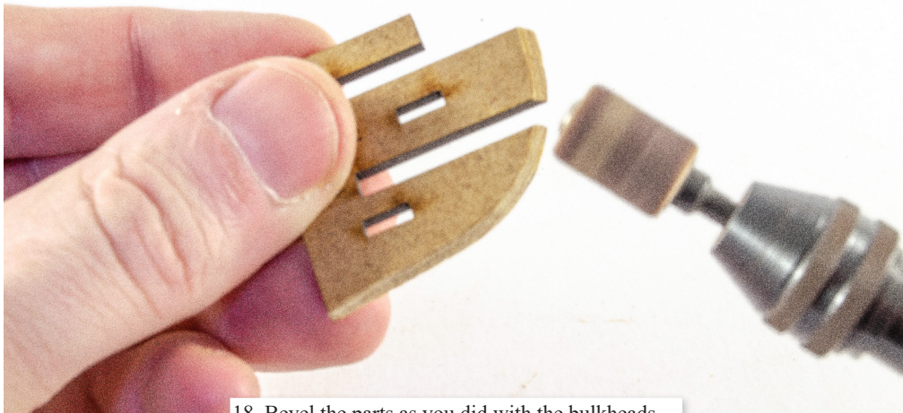
18. Bevel the parts as you did with the bulkheads.
