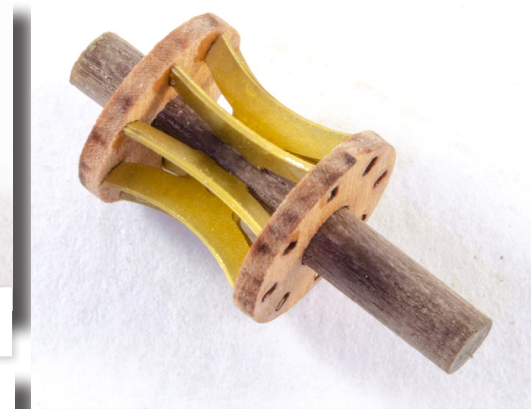
165. Now slot the other disc onto the other end and then sit the PE parts into the holes between the two, ensuring the holes are aligned on both discs. When you have all PE fitted, push the discs so the PE is properly trapped between them. Twist and adjust as necessary. Use a little CA on a cocktail stick and apply it to all joints.
