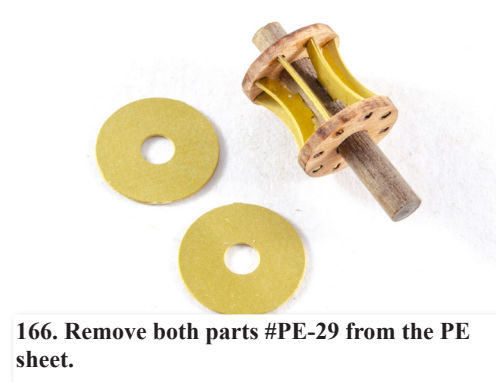
165. Now slot the other disc onto the other end and then sit the PE parts into the holes between the two, ensuring the holes are aligned on both discs. When you have all PE fitted, push the discs so the PE is properly trapped between them. Twist and adjust as necessary. Use a little CA on a cocktail stick and apply it to all joints.
