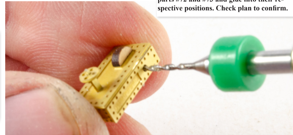
175. Use a 1mm drill bit to drill through the hole in the side of the assembly, and into the MDF.
