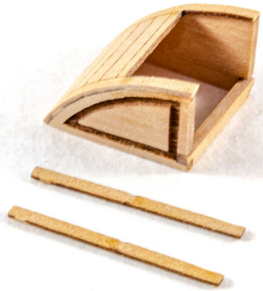
147. From the 0.6mm wood sheet, remove two parts #35.
