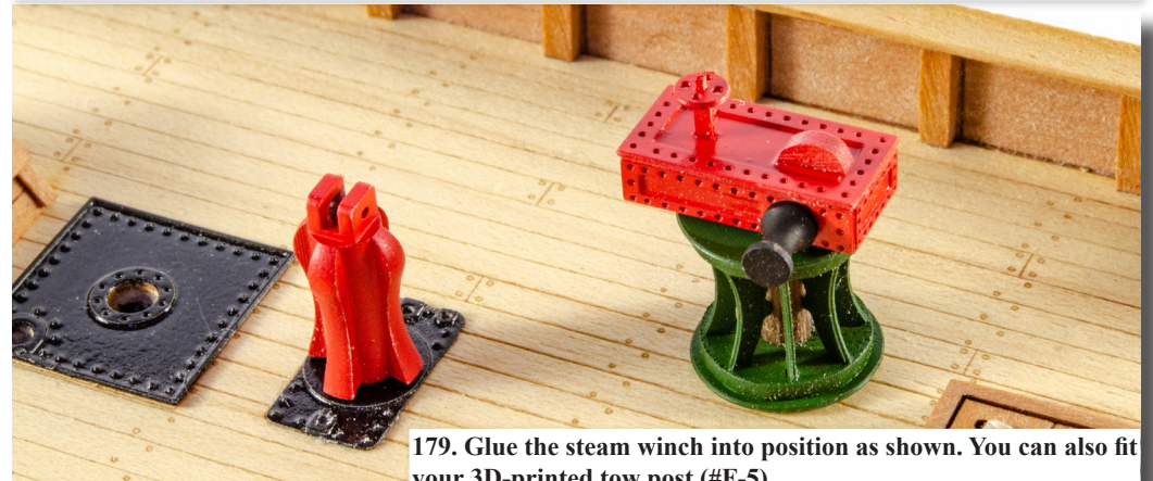
Paint the boiler plate (PE-24) and the smaller Tow Post Plate (PE-25) black and glue them into their respective positions on the deck
