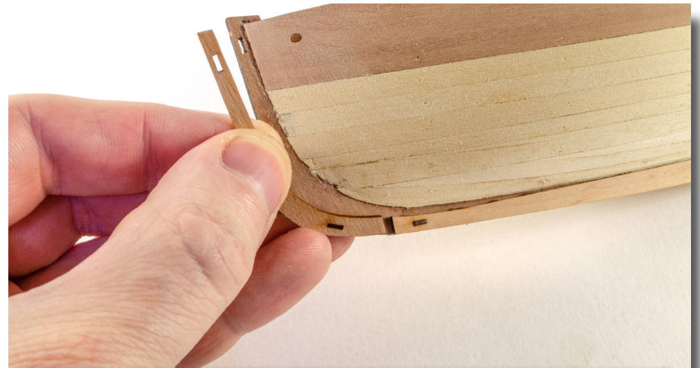
72. You will see how part #58 sits up against the stem of the model and the locating slots align.
