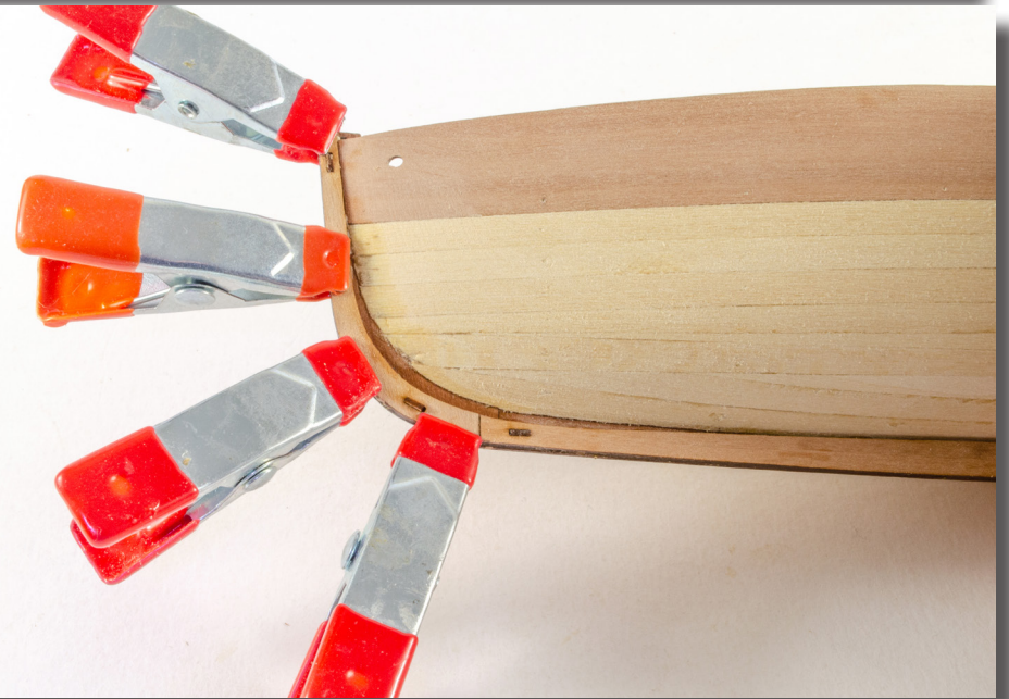
73. Glue part #58 into position and clamp. You can then fit the locating pegs through the parts and glue the other part #58 into position on the opposite side of keel.
