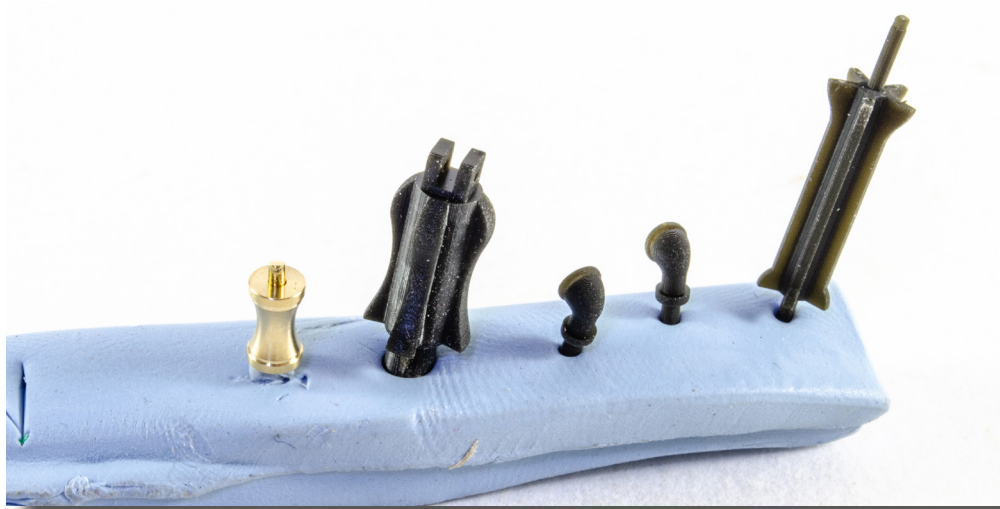
156. Take all your brass and 3D printed parts (not all shown here) and prime them before painting in your chosen colour. Our prototype used red paint.
