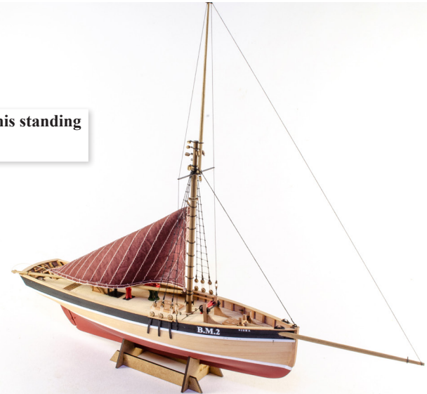
217. Before you can progress any further, you must add the shrouds, lanyards, and ratlines. These are a little tedious, but on Nisha, they are quick and straightforward to do. All this has to be done on the model. There are no tools to allow you to make them off model. We have included a paper template to help you with spacing. You can cut this from the plan and past to some card for rigidity.
