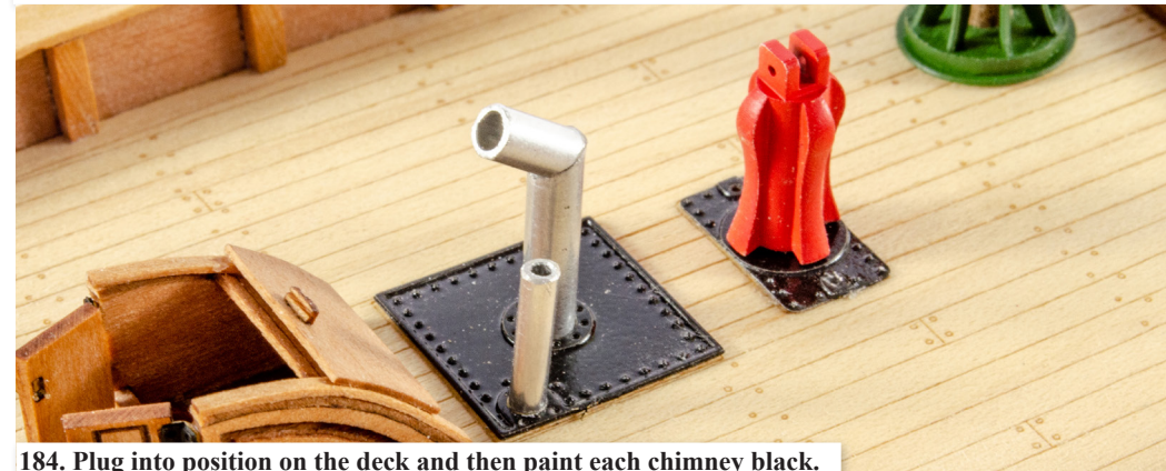
183. CHIMNEYS: Nisha was fitted with two chimneys. The small one is very easy to make. Simply cut a length of 2mm alloy tube, 39mm long and deburr the ends. The large chimney is made from 3mm tube. Cut the lengths as shown, with the adjoining angle, then use CA to glue the parts together. Made sure all parts are deburred.
