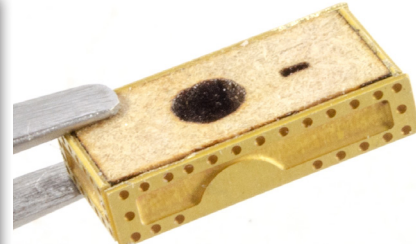
171. Now glue the side parts into position. These are parts #PE-31 and #PE-32. The orientation of these is very important. Use these photos and the plan to confirm you have this right. When complete, gently sand the top side of the assembly so it's totally level.
